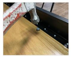
7 Open the bed, clear away any splintered wood and hammer in the T-Nuts in each hole.
