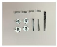
Needed: 1/4" Dill Bit, four T-Nuts, four 10-24 x 1/2" screws, two 10-24 x 1 3/8" screws Also Needed not shown: Drill,
