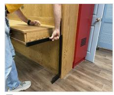
3 Close bed and remove screws at the pivot point on both sides using an allen wrench. Have a helper hold the desk. It could pull the face open.
