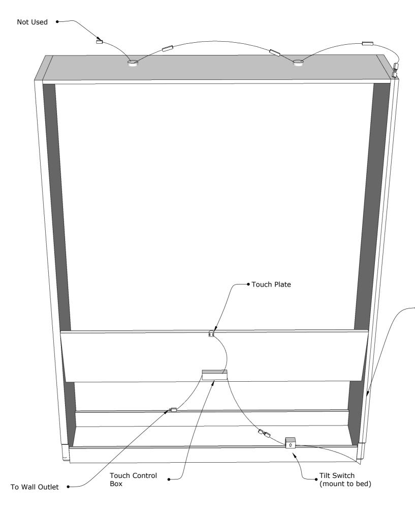
Cord connected to • Tilt Switch running up the Vertical.
